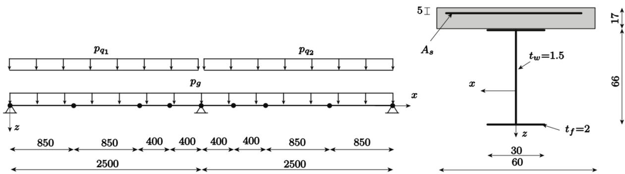
Figure 4. Continuous girder disposition (left) and composite cross section (right). Units: [cm].
