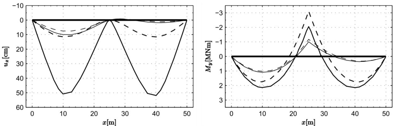
Figure 5. Vertical displacements (left) and bending moment (right): LC1 plastic (—), LC1 elastic (---), LC2 plastic (-.-), and LC2 elastic (....).
