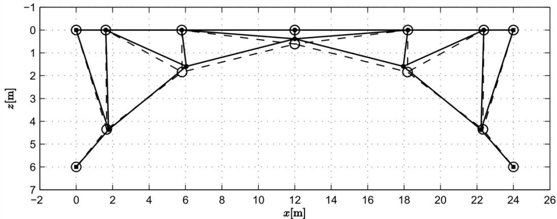
Figure 8. Comparison of truss bridge optimal shape: this work (-●-), Soh&Yang (-○-).
