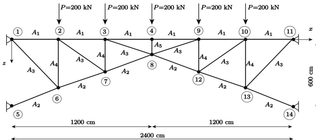
Figure 7. Truss bridge. Units: [cm]; [kN].
