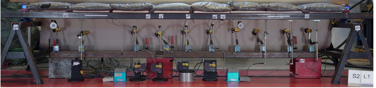
Figure 8. Experimental set-up: deflection, inclination and strain sensors are installed in a simply-supported steel beam. A static load uniformly distributed is applied with bags of steel spheres, resting on wooden plates.
